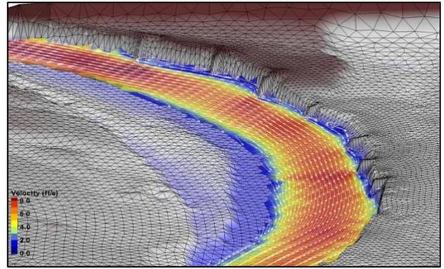
SMS's SRH-2D model is appropriate for most transportation and fish passage hydraulic applications because it incorporates 2D hydrodynamic routing; steady and unsteady detailed 2D channel and floodplain modeling; while also modeling local flow velocities, eddy patterns, flow recirculation, lateral velocity variation, and flow spills over banks and levees; and illustrating flood mapping and flood animations (such as velocity vector tracing).
