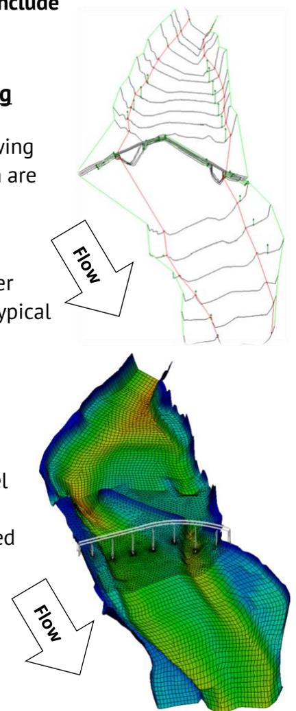
Figure 1. (Top graphic) 1D model output - The channel geometry is represented by, and the hydraulic computations occur at, each cross section. (Bottom graphic) - 2D model output - The channel geometry is represented by thousands of elements, and hydraulic computations occur at each element. Source: Rick Macala, CDFW.
